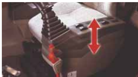
Independently adjustable control module height
